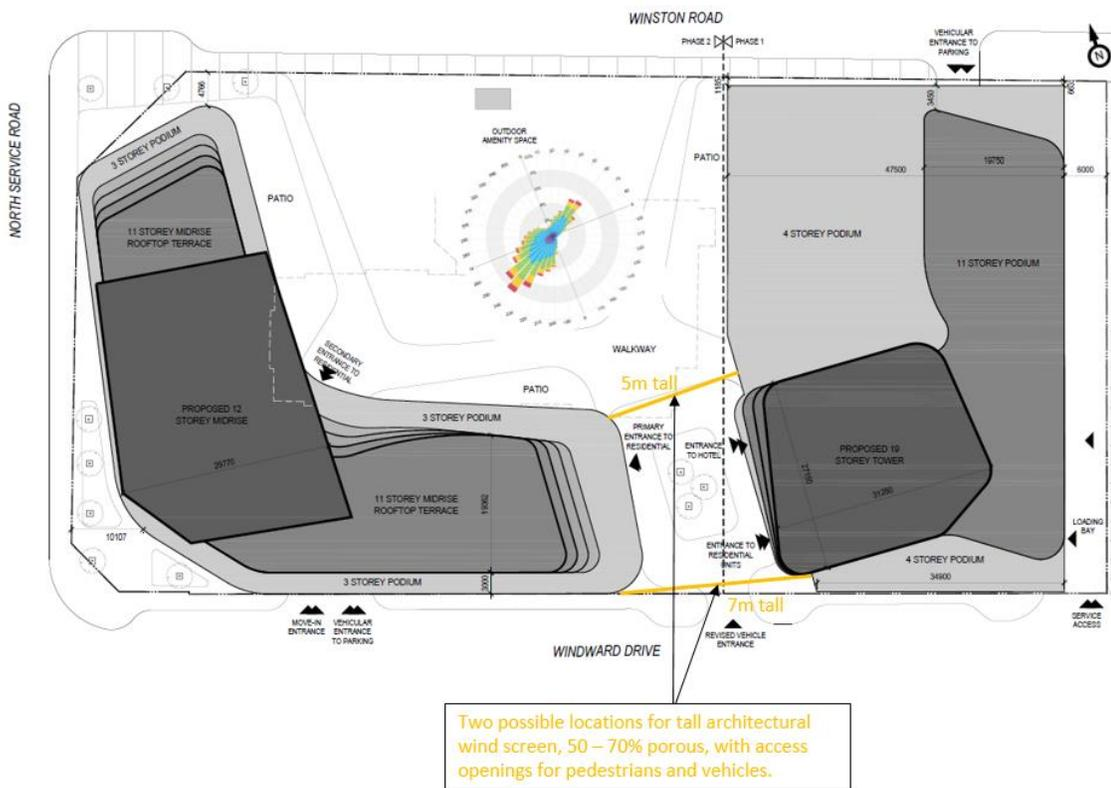
Image 5: Proposed Site Plan Showing Entrance Locations and Wind Control Concept
